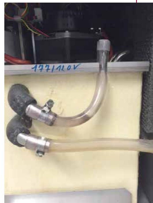
Contamination can be seen in the dark area of a heater-cooler device tube. Photo provided by Keith Allen, MD.
